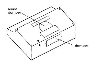
Attach rectangular damper to selected rectangular vent opening. If damper is attached to back of range hood, be sure damper hinge is toward the top. For round vented installations, use round damper in duct to prevent air from flowing back into ductwork. If wall or roof cap has a damper, remove damper blade from range hood.
